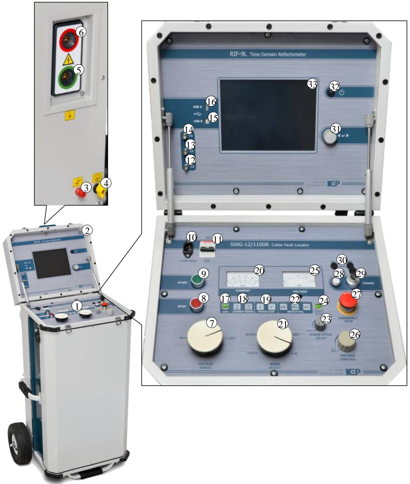
Figure 1 – Design and layout of user controls and connectors of System
